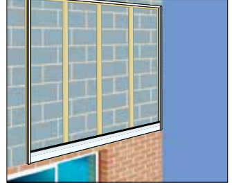
3. Fit first plank at base
